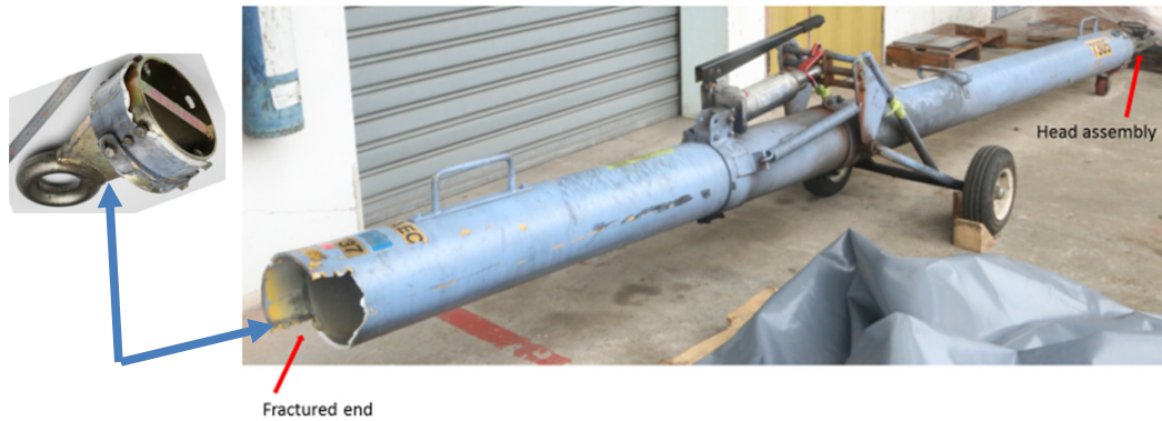
Figure 5: Damage to towbar
