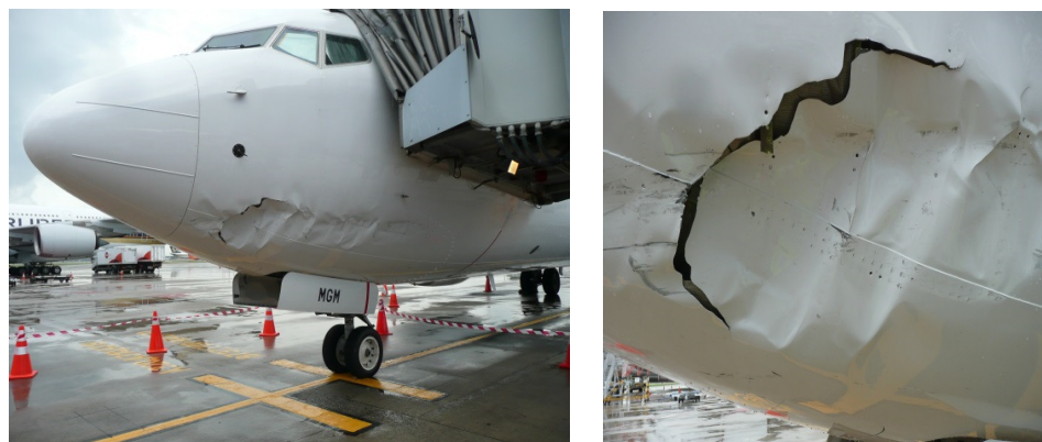
Figure 4: Damage to the lower left front fuselage
