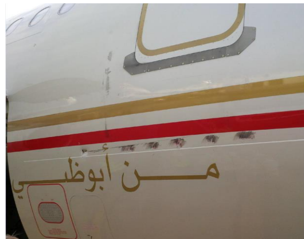
Figure 4. Damage to fuselage – dents
