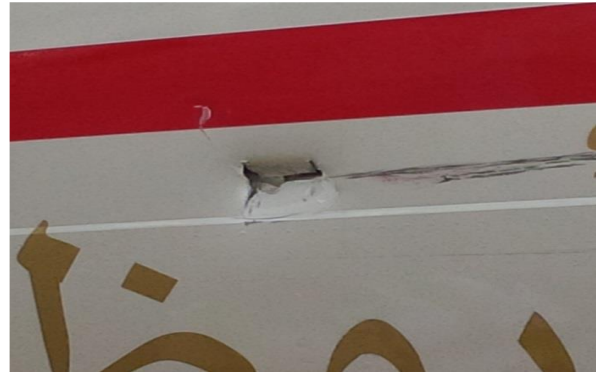
Figure 3. Damage to fuselage – skin puncture
