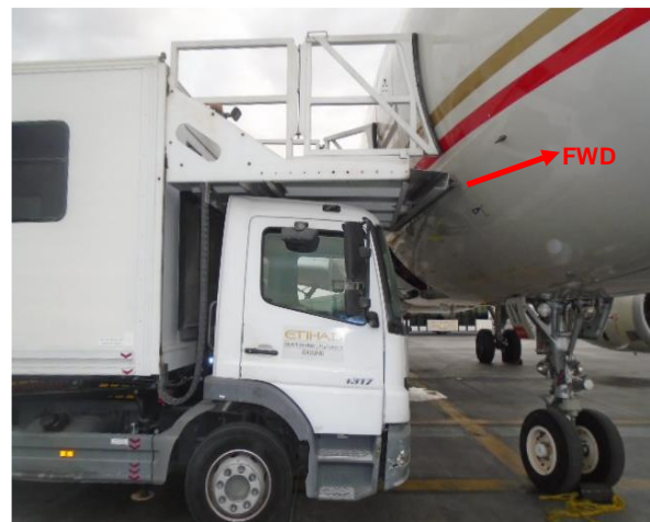
Figure 1. MHL collided with the Aircraft at R1 door
