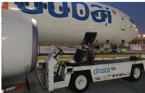
Figure 1. The MCB in contact with the engine. The MCB was parallel to the Aircraft
