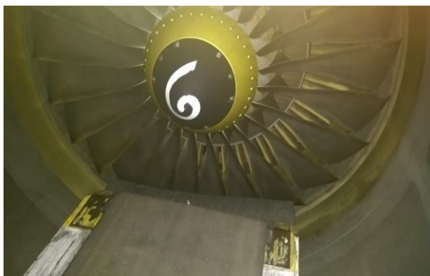
Figure 2. Final position of MCB inside engine inlet damage
